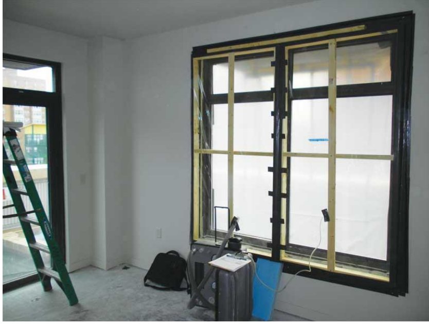
Hava kaçak testi (ASTM E783)
